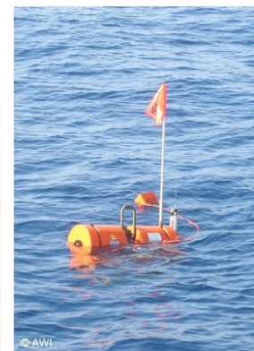
Ocean bottom seismometer in the Aegean Sea.
